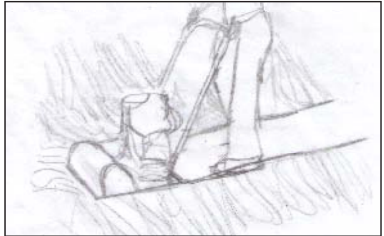
Compacting the sand with a mechanical compactor
